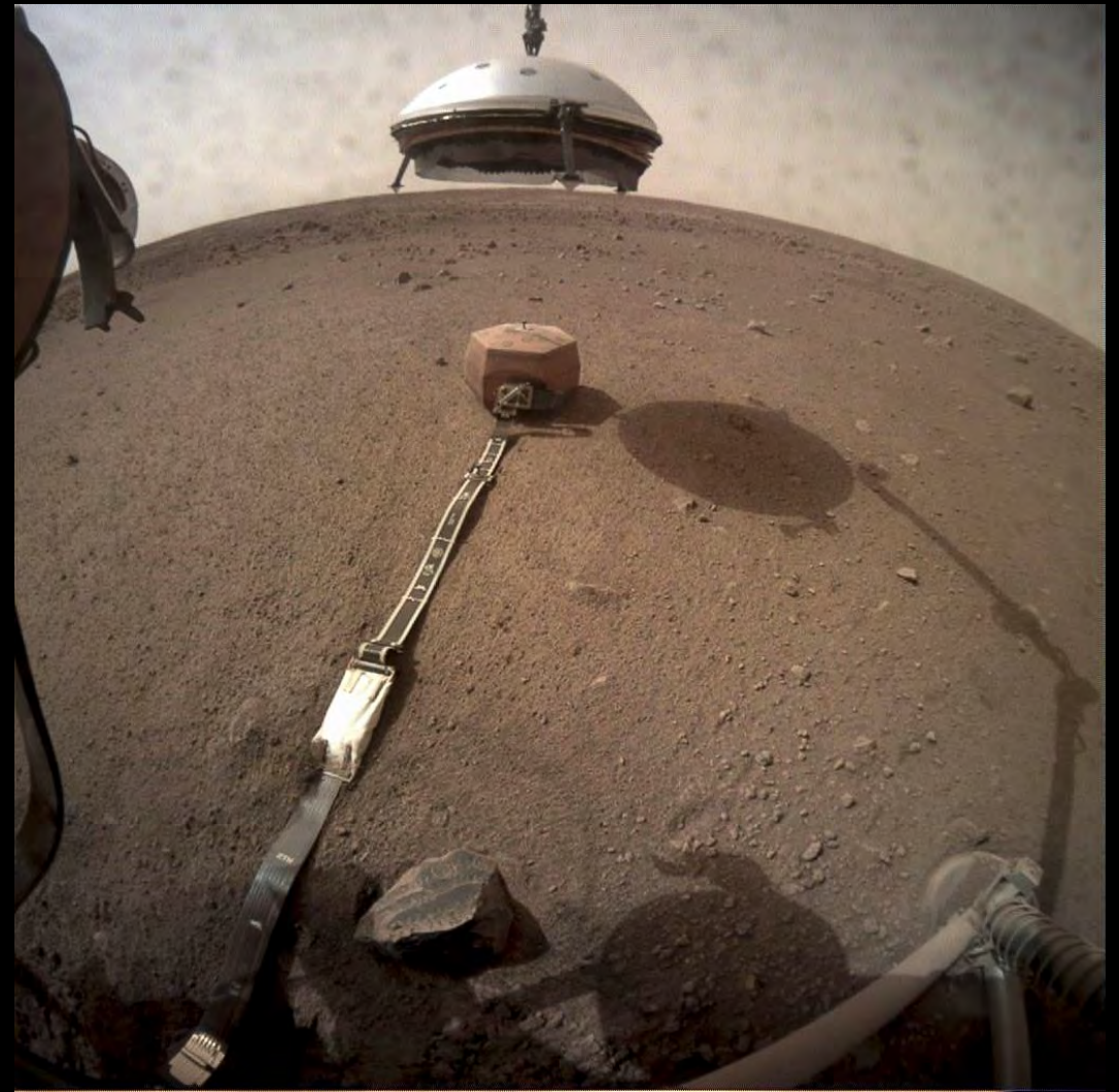
SEIS seismometer deployed on Mars with its shield overhead ©NASA/JPL Caltech 2019
